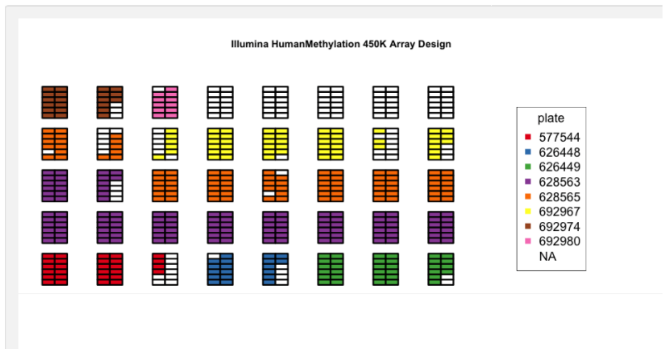
Figure 2: Array design panel The plot represents the physical slides ( 6 \times 2 samples) on which the samples were assayed in the machine. The user can select the phenotype to color the samples. This plot allows to explore the quality of the randomization of the samples for a given phenotype.
