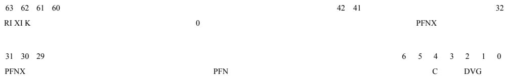
FIGS 7-3 EntryLo0 and EntryLo1 in DMFC0 / DMTC0 instruction format accessible register
