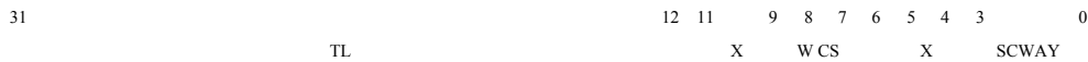
Figure 7-50 The format when the TagLo register is used to access the D-Cache Tag
