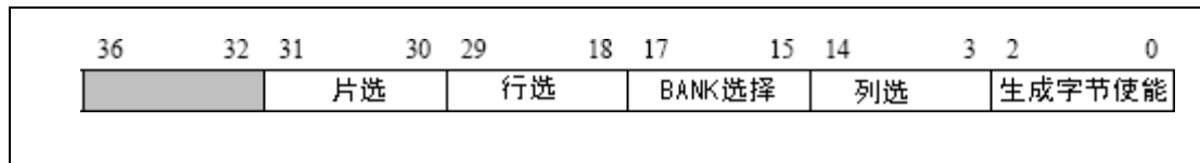
Figure 8-1 DDR2 SDRAM column and column address and CPU physical address conversion
